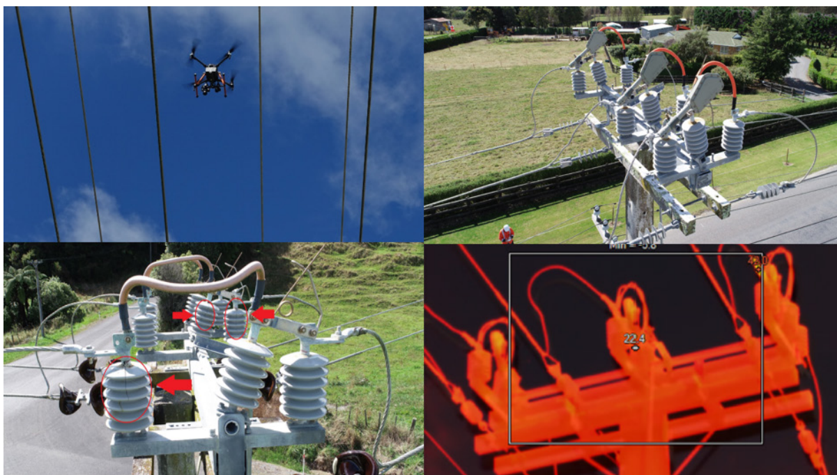
Figure 4-15: Continued improvement of condition-based risk monitoring of assets using UAV drone inspections and thermal imaging
