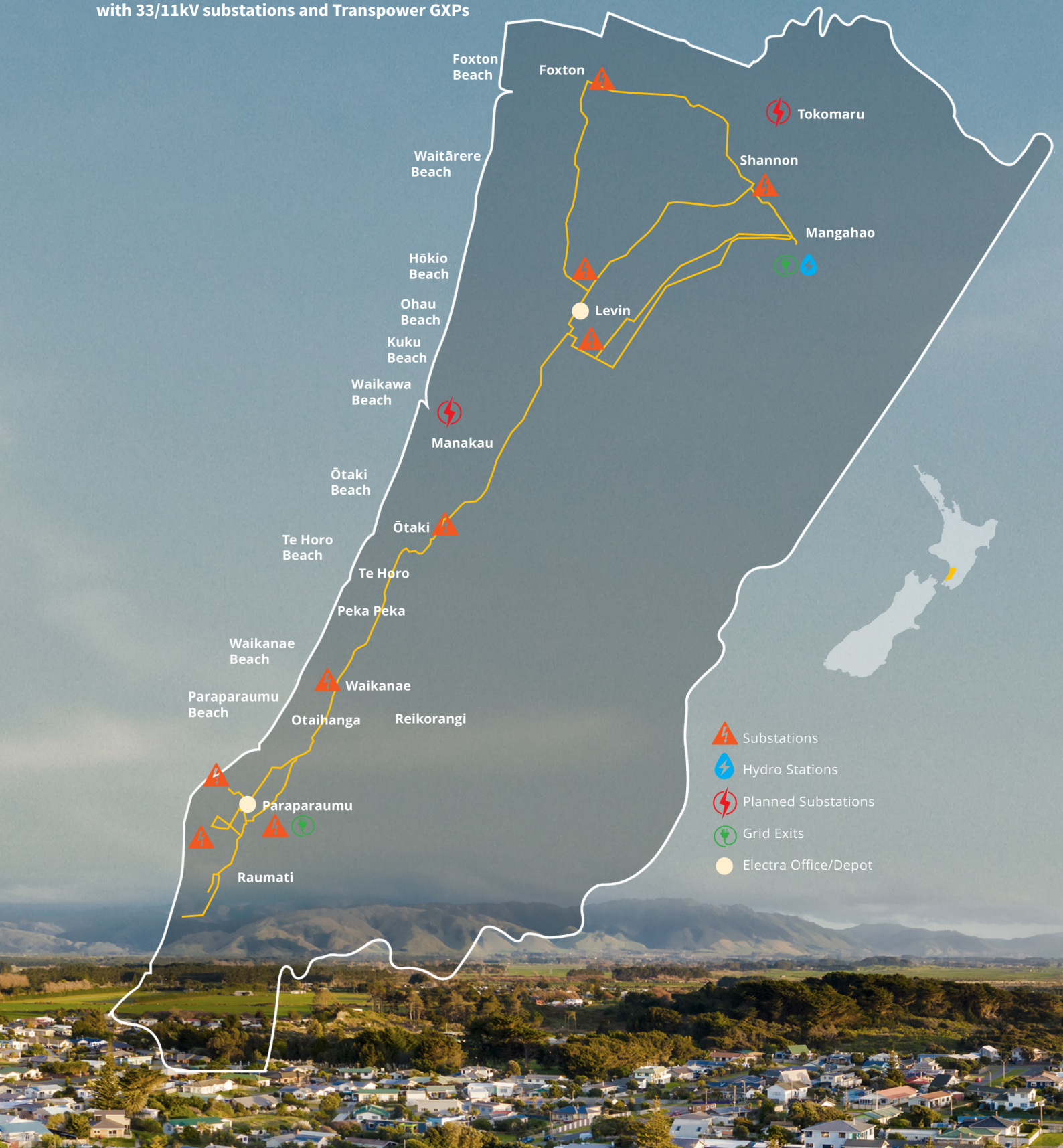
Figure 2-1: Electra sub-transmission 33kV network with 33/11kV substations and Transpower GXP
