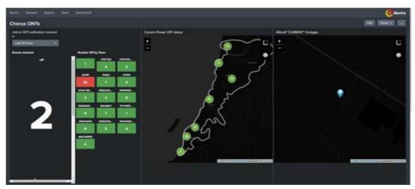
Figure 2-6: Splunk dashboard indicating power loss on Chorus optical fibre connections
